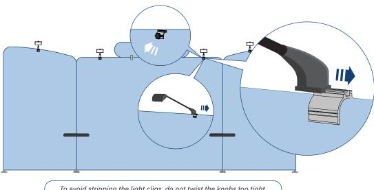
To avoid stripping the light clips, do not twist the knobs too tight.
